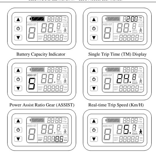
In display interface, if you hold button (SW) long, the meter will be powered-off together with that of the controller.
