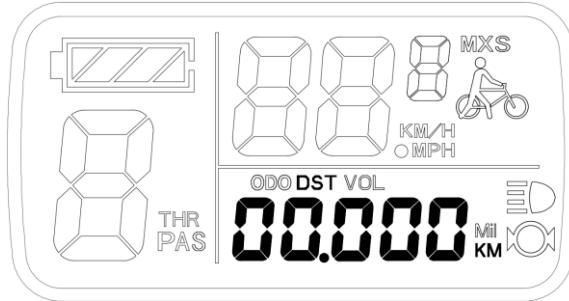
**Under the status of data flashing, if there were no operations on the data within 5 seconds, the meter will automatically return to display1 after 5 seconds, and the original record content will be saved.**
