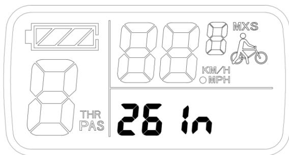
**Under the wheel diameter setting interface, if there's no button operation on the meter for more than 1 minute, and then the meter will automatically return to display 1, and the original set values will be saved.**
