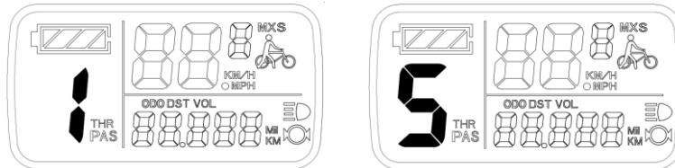
**At every startup, the meter will automatically restore gear (this can also be configured as required by users) when it was at last shut down. When the power assist ratio is gear 0 zero, there's no power assist function.**
