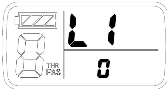
After finishing L1 parameter setting, press **[①]** button (**SW**) to save the current value and then enter L2 parameter setting interface.
