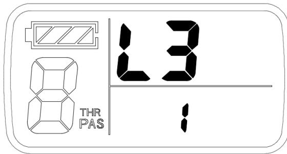
After finishing L3 parameter setting, hold [SW] button (SW) for about 2 seconds to exit L parameter setting environment and return to the display 1.
