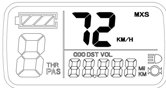
**Under the setting maximum riding speed interface, if there's no button operation on the meter for more than 1 minute, and then the meter will automatically return to display 1, and the original set values will be saved.**
