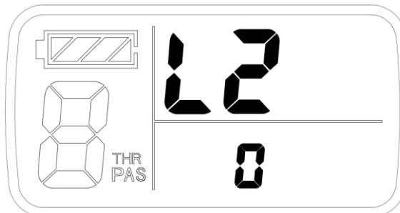
After finishing L2 parameter setting, press **[①]** button (**SW**) to save the current value and then enter L3 parameter setting interface.
