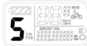
Power Assist Ratio Gear (ASSIST)
