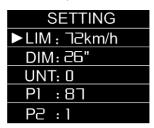
Within 5 seconds after power on, hold and at the same time to enter General Setting interface, move to maximum speed setting, press button maximum riding speed flash, press or to set the maximum riding speed (default 25Km/H).
